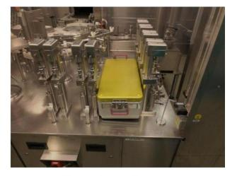
No stopper container → Operator leans over hopper during re-fill
