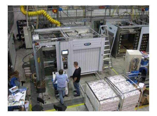
Cycle development tests using actual production unit and sample loads => Initial optimization and parameters to benefit the final validated cycle
